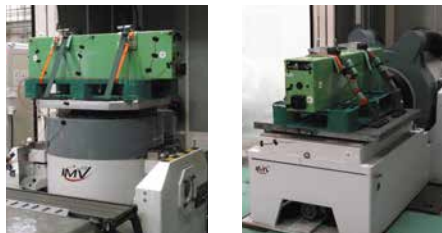
JIS Z-0200JIS Z 0200 UN38.3 TestT.3Vibration(38.3.4.3.2) 2.5.7 Vibration Test based on Development of Energy Storage System for Grid-connection with Renewable Energy Resources —Basic research for the fundamental study by NEDO
