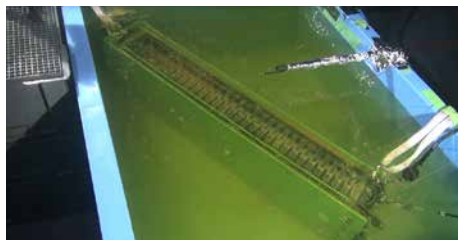
2.5.9 Immersion Test based on Development of Energy Storage System for Grid-connection with Renewable Energy Resources —Basic research for the fundamental study by NEDO
