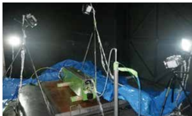
Battery for power storage system(JEAC 5006-2010) table 3-6-2 in Articles 3 to 6 2.5.3 Overcharge test based on Development of Energy Storage System for Grid-connection with Renewable Energy Resources —Basic research for the fundamental study by NEDO
